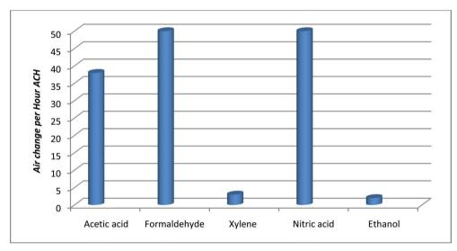
Figure 2. Air change per hour to reach PEL level in 100 m<sup>3</sup>.
