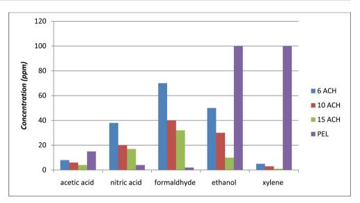
Figure 1. Concentration from evaporation of 1 m<sup>2</sup> of liquid spill in 100 m<sup>3</sup> space.
