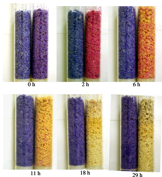
Figure 6. Oxygen depletion in GCR using Resazurin as an indicator. Images were taken at specific intervals (0, 2, 6, 11, 18, 29 h) for control (without inoculation, left reactor) and experimental (with inoculation, right reactor) columns.
