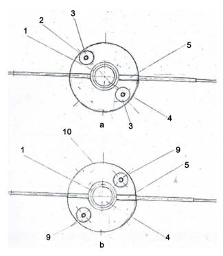
Figure 4. Location of electrorocket engines of forward and backward movement.
