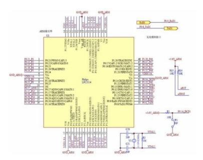
Figure 4. ARM Interface Circuit
