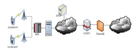
Figure 1. GPRS Principle Structure Diagram
