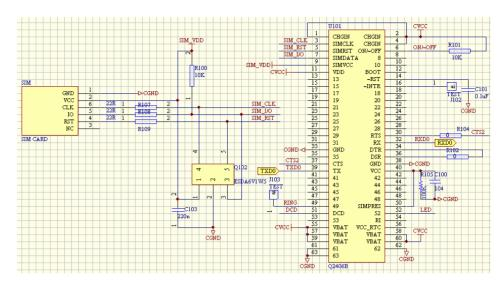
Figure 5. GPRS Module Interface Circuit
