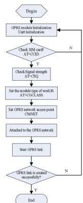
Figure 6. Flowchart of Establish GPRS Links
