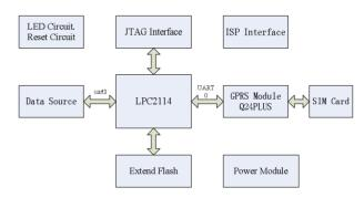
Figure 3. Block Diagram of the Hardware
