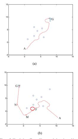
Figure 2. Simulating effects of improved obstacle avoidance algorithm based on the artificial potential field
