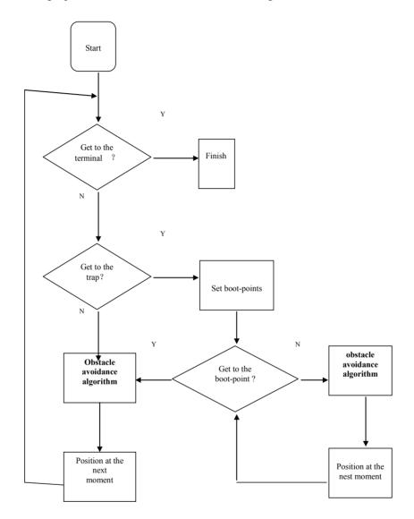
Figure 1. Setting boot-point algorithm
