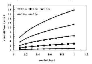
Figure 3. Conduit flow corresponding to conduit head and diamater
