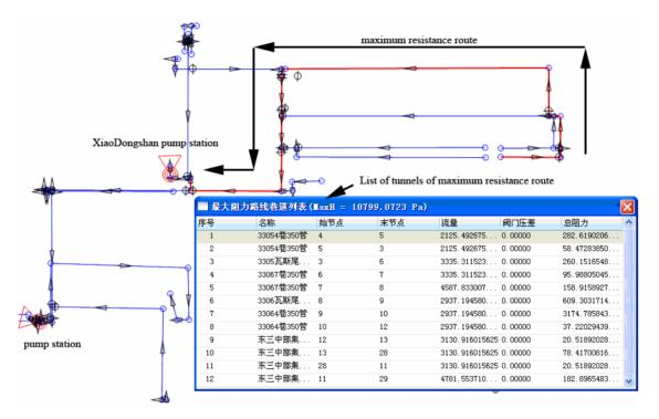
Figure 3. The resistance route diagram of Third East Area after when the XiaoDongshan pump station is built
