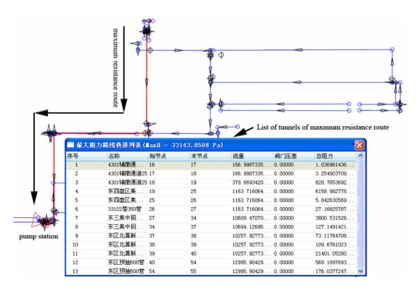
Figure 2. The diagram of maximum resistance route of pumping pipeline system
