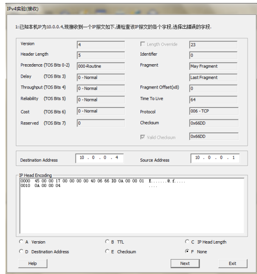
Figure 1. IP data packet fields accuracy test example
