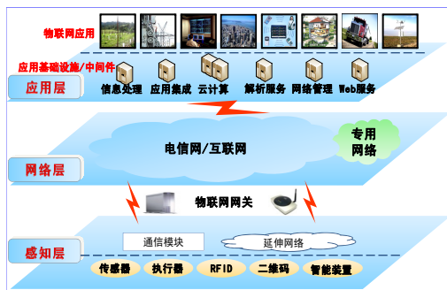
Figure 2 Things Smart Grid Architecture 图 2 智能电网物联网体系架构
