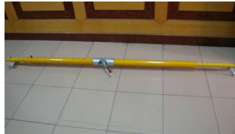
Figure 2. Line shape of insulating supporting stick 图 2. 一字形支杆
