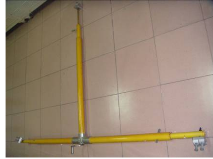
Figure 1. Triangular shape of insulating supporting stick 图 1. 三角形支杆
