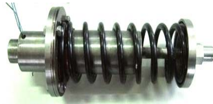
Figure 2 MR shock absorber developed independently 图 2 自行研制的双出杆磁流变减振器
