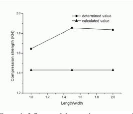
Figure 4. Influence of base ratio on compression strength of boxes with height of 30 cm and perimeter of
