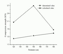
Figure 2. Influence of perimeter on compression strength of boxes with height of 40 cm and base ratio of 1.5.
