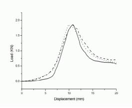
Figure 1. Load vs. displacement curves for three boxes with length of 360 mm, width of 240 mm and height of 300 mm respectively.
