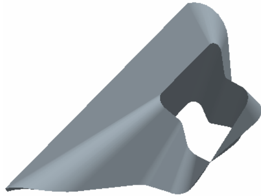
Figure 5. 3-D Model of shoulder with butterfly section.
