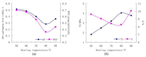
Figure4. Effect of heating temperature on main packaging properties of WPC film
