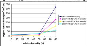
Figure 3. Oxygen transmission rates of solvent cast pectin films (100  $\mu$ m) with different amounts of nanoclay.
