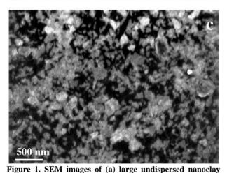
aggregates. The excerpt shows the surface structural features: laminar fine structure can be seen on the aggregate surfaces, (b) spincoated nanoclay platelets after dispersing with the ultrasonic microtip, and (c) spincoated nanoclay platelets after high pressure fluidizer treatment.
