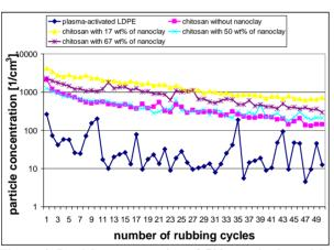
Figure 4. Particle concentration of 500 nm sized particles in air during rubbing of different coatings
