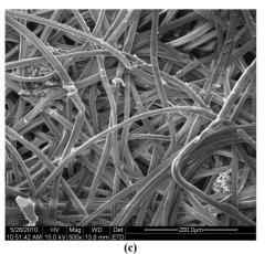
Figure 1. SEM micrograph (a) chitosan microsphere; (b)&(C) the surface of nonwovens with microspheres containing levofloxacin
