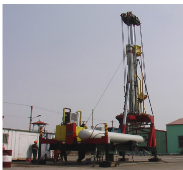
Figure 1. Hydraulic energy-storing workover rig 图 1 液压蓄能修井机
