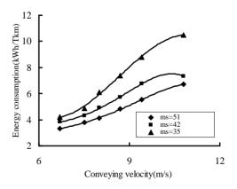
Figure.4 Trend of energy consumption in different conveying velocity
