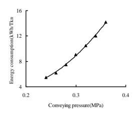
Figure.3 Trend of energy consumption in different conveying pressure
