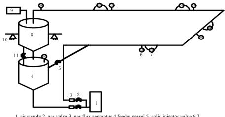
1. air supply 2. gas valve 3. gas flux apparatus 4.feeder vessel 5. solid injector valve 6,7. static/differential pressure cell 8 receiver vessel 9dust collector 10. weight balance 11. balanced valve **Figure.1 Schematic diagram of experimental system**
