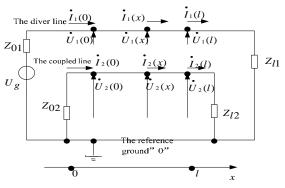
Figure 4 Equivalent circuit of voltage and current relations
