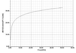
Figure 9 Relationship of signal attenuation parameters and frequency
