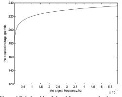
Figure 6 Relationship of signal frequency and voltage gain
