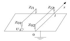
Figure 1 Two-wire transmission line model in PCB design
