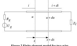
Figure 2 Finite element model for two-wire
