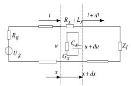
Figure 3 Equivalent circuit model of two wire
