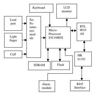
Figure 1. System hardware schematic structure
