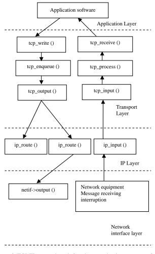
Figure 3. TCP/IP protocol stack function organization structure of LWIP
