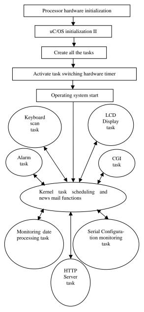
Figure 2. System software flow chart
