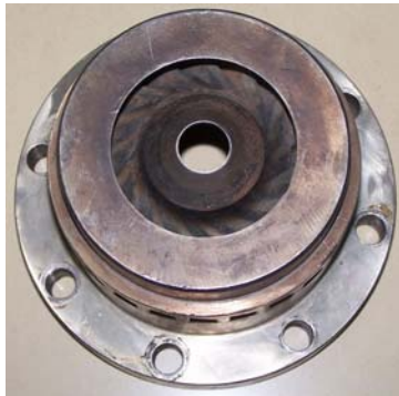
Figure 2. Radial swirling nozzle
