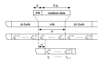
Figure 1. Frame synchronization model<sup>[5]</sup>
