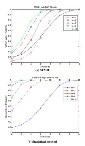
Figure 6. Effect of frame number M on detection performance
