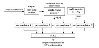
Figure 2. Schematic diagram of multiple-frame detection using statistical method
