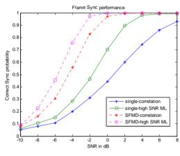
Figure 3. Comparison of SFMD and single-frame detection
