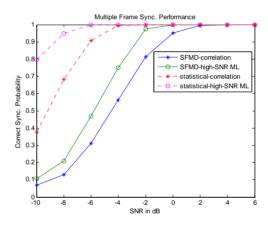
Figure 5. Comparison of the two multiple-frame detection method
