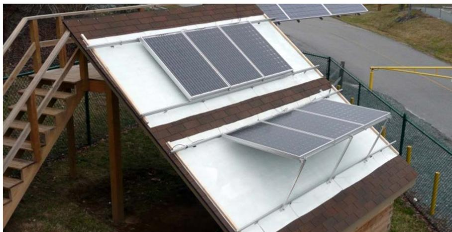
Figure 7. Photo of Trial 3. Lower array poised at horizontal. Upper array white TIOCOAT™-3 modules, lower array white TIOCOAT™ 3 modules horizontal. (Refer to Table 1 for details).
