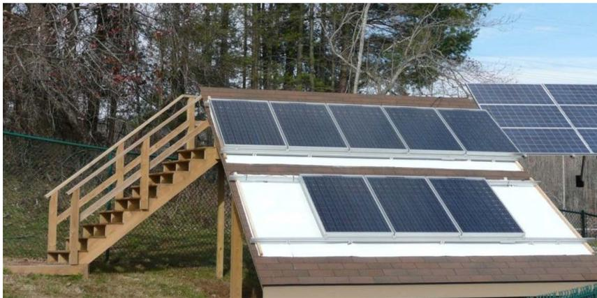
Figure 4. Photo of Trial 2. Upper array white TIOCOAT™ Flush 5 modules, lower array white TIOCOAT™ Flush 3 modules. (Refer to Table 1 for details).
