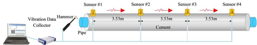
**Figure 7.** Schematic diagram of steel pipe concrete knockdown test.
