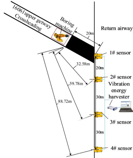
**Figure 10.** Diagram of underground boring vibration test sensor arrangement.
