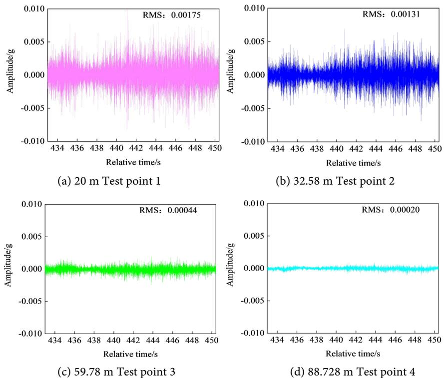
**Figure 11.** Time domain waveforms at each measurement point for underground boring vibration test 3.
