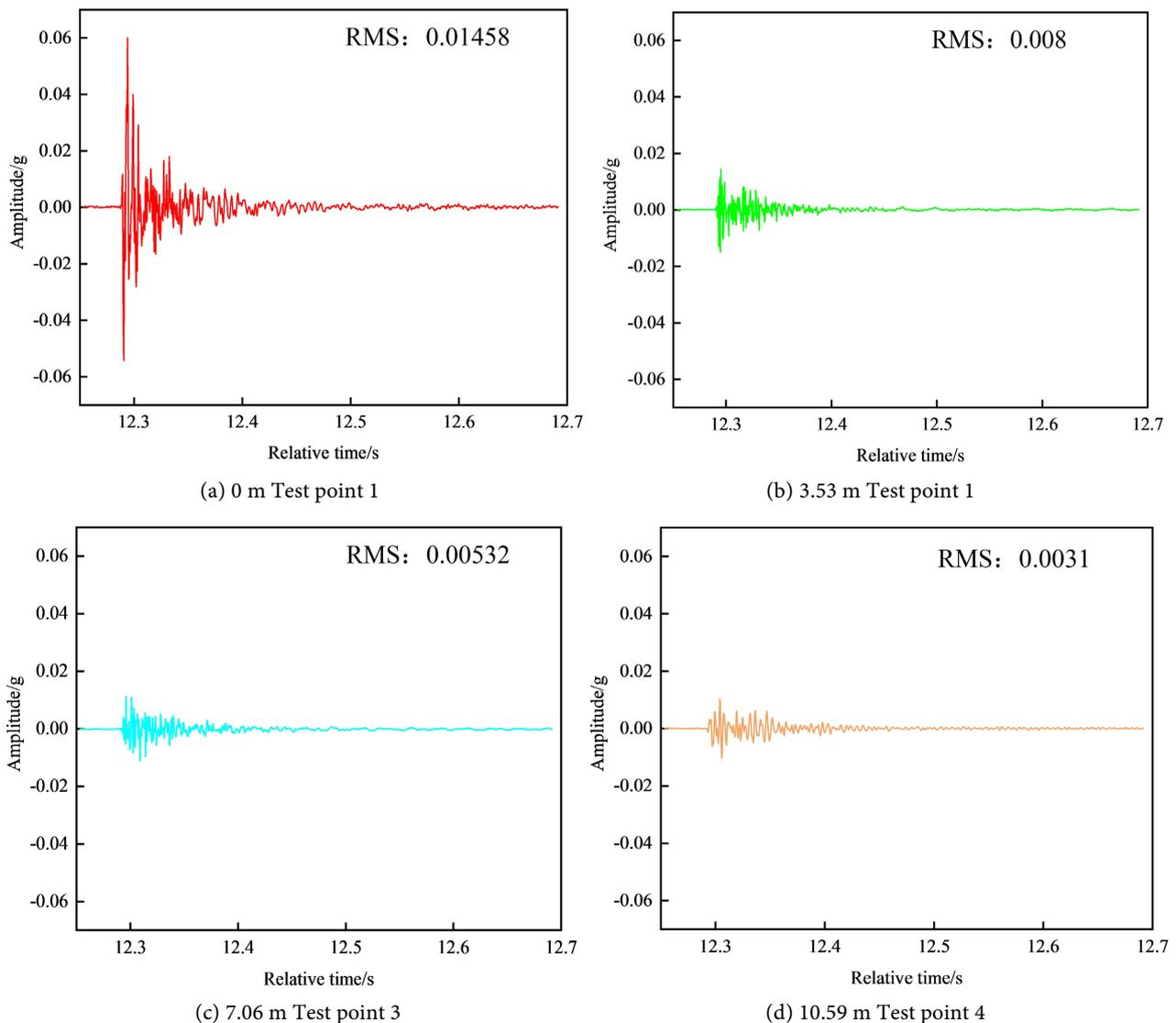
**Figure 8.** Vibration time domain acceleration amplitude at each measurement point of group A of steel pipe concrete vibration test.
