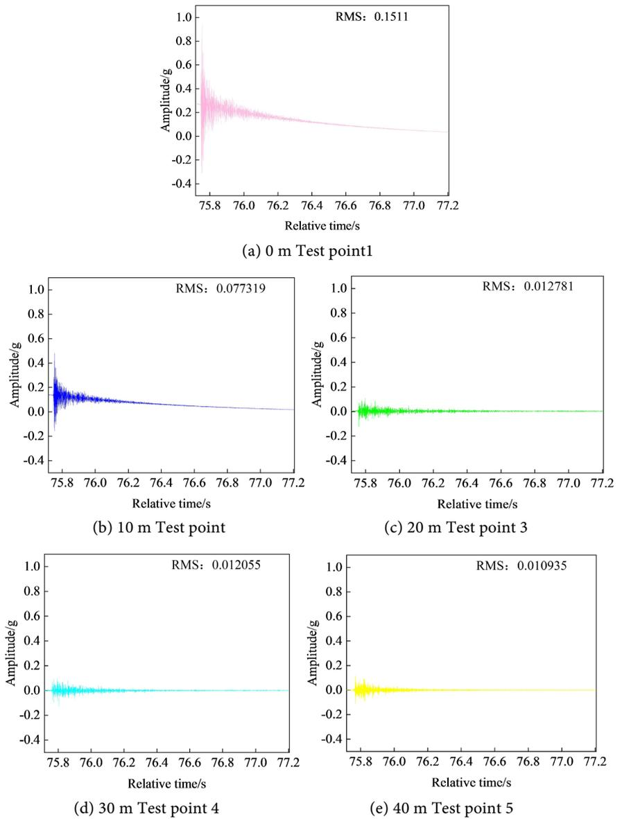
**Figure 5.** Steel pipe vibration test 1 time domain waveforms at each measurement point.
