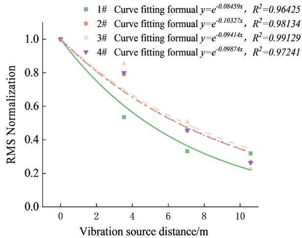
**Figure 9.** Root mean square normalized exponential decay fitting curve.
