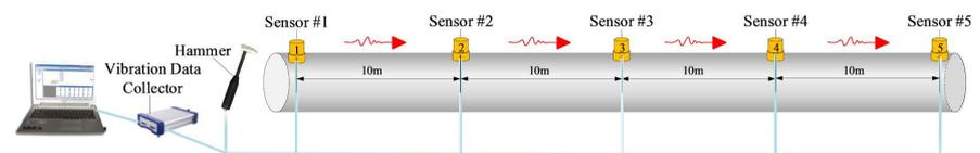
**Figure 4.** Schematic diagram of the steel tube vibration test.
