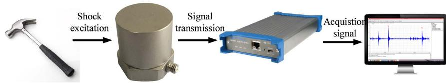
**Figure 3.** Vibration test system framework.
