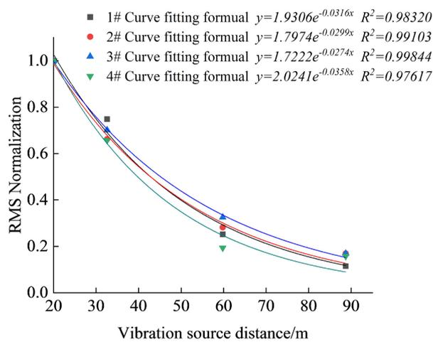
**Figure 12.** Fitting curve of root-mean-square relative value index of 1 - 4 groups of underground driving vibration.
