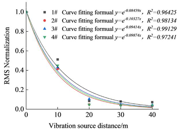
**Figure 6.** Fitted graph of the root mean square relative value index for steel tube vibration groups 1 - 4.
