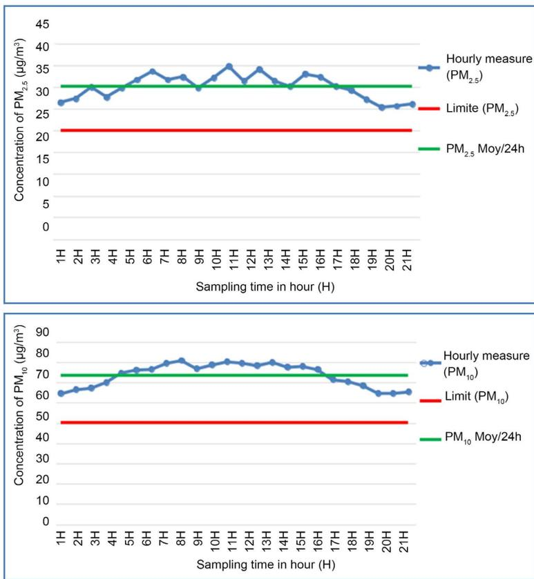
Figure 5. Variation of PM<sub>2.5</sub> and PM<sub>10</sub> dust TONGON.
