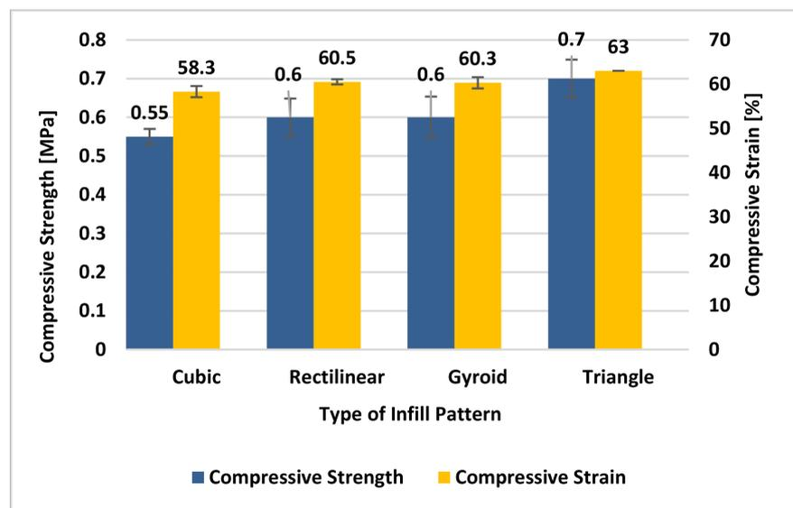
**Graph 6.** Comparison of compressive strength and compressive strain with 25% infill.
