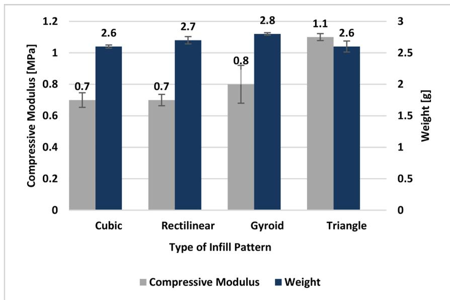
Graph 3. Comparison of compressive modulus of different patterns with 25% infill.
