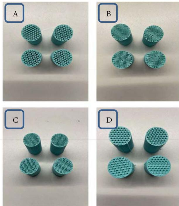
**Figure 5.** Infill patterns ((A) Triangle, (B) Rectilinear, (C) Gyroid and (D) Cubic).
