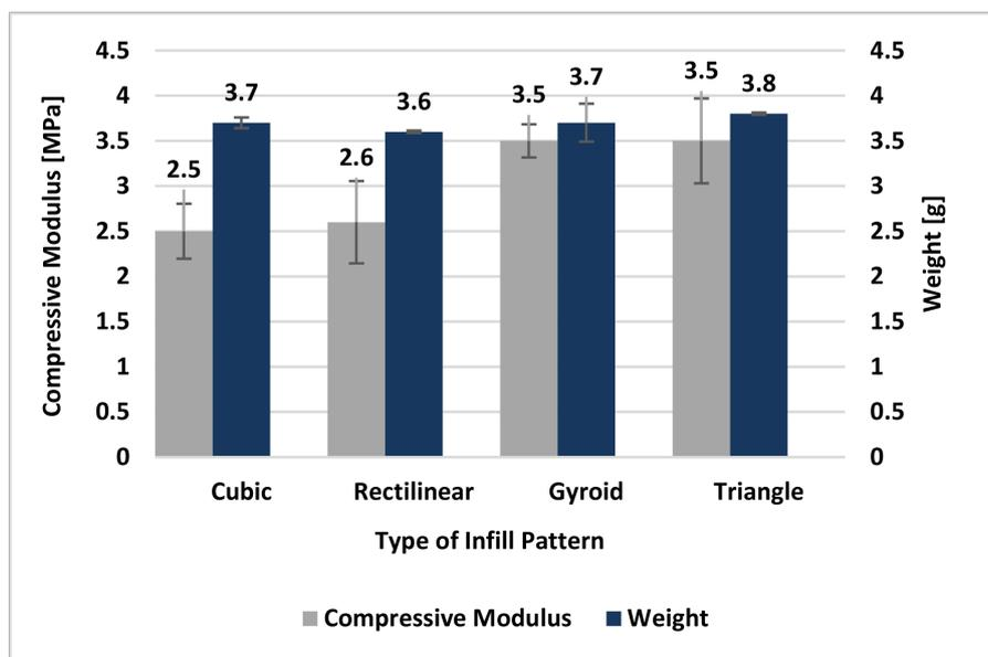
Graph 2. Comparison of compressive modulus of different patterns with 40% infill.
