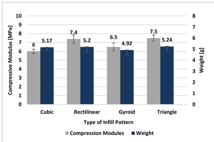
Graph 1. Comparison of compressive modulus of different patterns with 60% infill.
