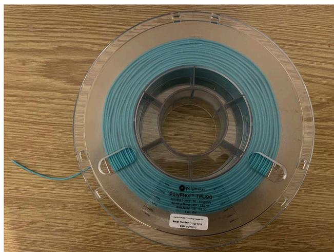
**Figure 2.** TPU filament.
