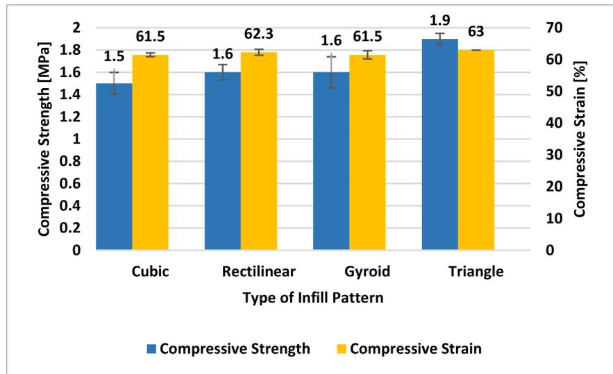
**Graph 5.** Comparison of compressive strength and compressive strain with 40% infill.
