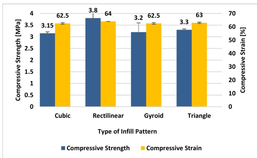
Graph 4. Comparison of compressive strength and compressive strain with 60% infill.
