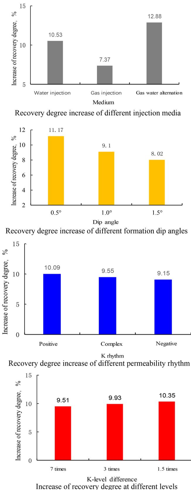
**Figure 4.** Orthogonal experimental results of recovery degree of residual oil at the edge of 943 sand body.
