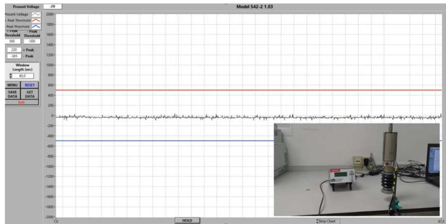
**Figure 6.** Monitoring charge accumulated in surface using Trek Voltmeter 542A-2.
