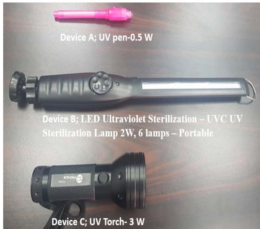
**Figure 2.** Three UV light tested for their ability to kill Bacteria or Viruses.
