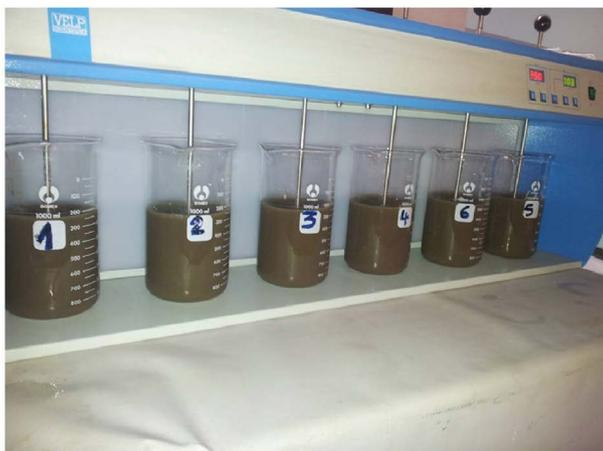
**Figure 2.** Jar-test device.
