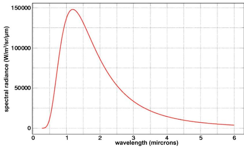
Figure 11. Probability distribution of the radiations emitted from 100 watt filament bulb.
