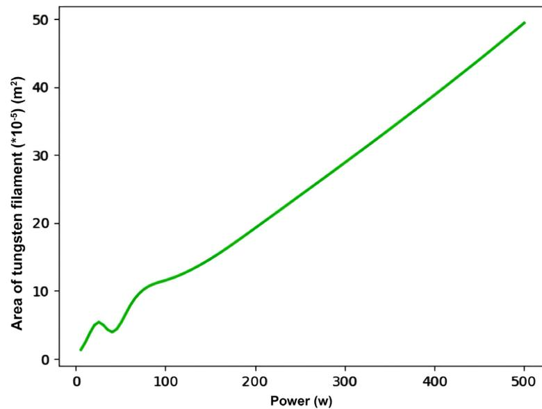
**Figure 8.** Dependence of power of bulb with surface area of the filament.
