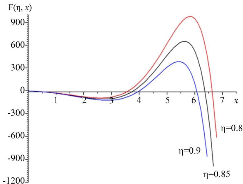
**Figure 4.** Spectrum curve of the blackbody thermal radiation [18].
