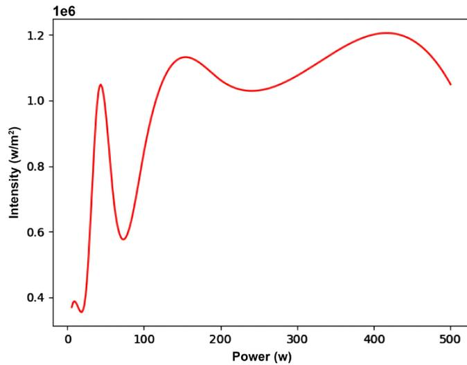
**Figure 5.** Dependence of intensity of radiations on power of the bulb.
