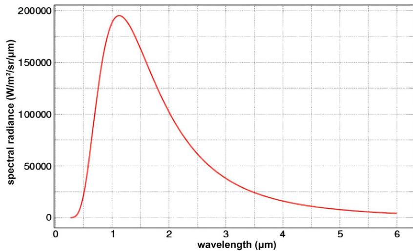
Figure 12. Probability distribution of the radiations emitted from 500 watt filament bulb.
