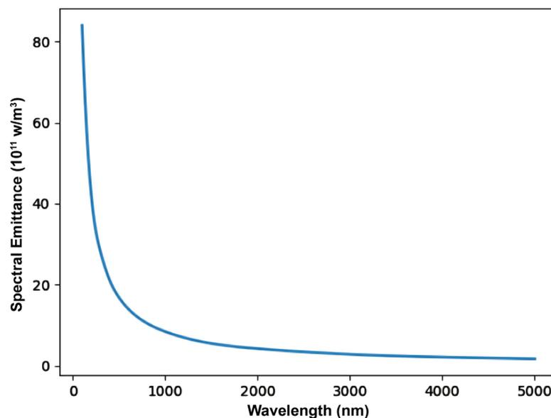
**Figure 9.** Dependence of spectral emittance on the wavelength.
