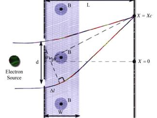
Figure 2. (Color online): The standard double-slit apparatus with an additional strip of a perpendicular magnetic field B of width W placed between the slit-region and the observation screen. In the text we deal for simplicity with the case  $W \ll L$  so that deflections (of the semiclassical trajectories) due to the Lorentz force, shown here for a negative charge q, are very small.
