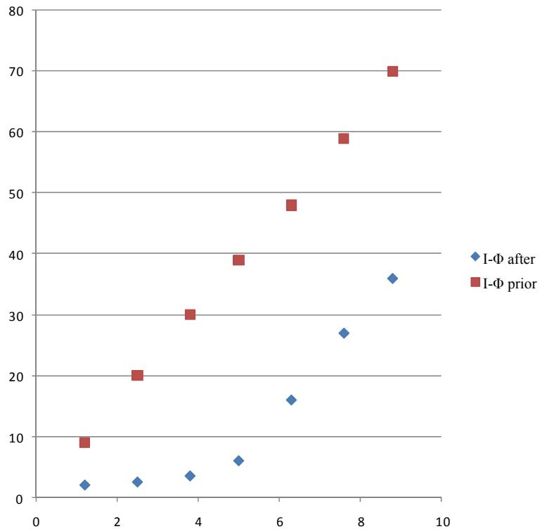
**Figure 1.** Representative Si p-i-n photodetector optoelectronic-response I-Φ experimental characteristic ( $I$  in  $\mu\text{A}$ , IR at  $\lambda = 780 \text{ nm}$   $\Phi$  in  $\times 10^{15} \text{ photons}/(\text{cm}^2 \cdot \text{s})$ ) monitored prior to (upper marks) and after (lower marks) the photodiode's exposure to a cumulative  $\alpha$ -particle dose of  $3.8 \times 10^{10} \alpha\text{-particles}/\text{cm}^2$ , well above the pertinent threshold.
