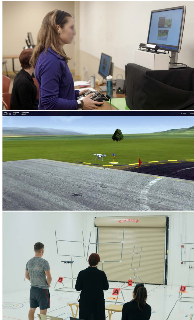
Figure 1. Experimental tasks. Top panel: participants viewed instructional flight videos while holding UAS controllers and mimicking movements in the video task. Center panel: participants controlled a virtual UAS in a number of flight tasks within Real Flight 7.5 software as part of the simulation task. Bottom panel: participants controlled a UAS through a series of physical obstacles as part of the live flight task. Depicted participants provided written informed consent for publication of this figure.
