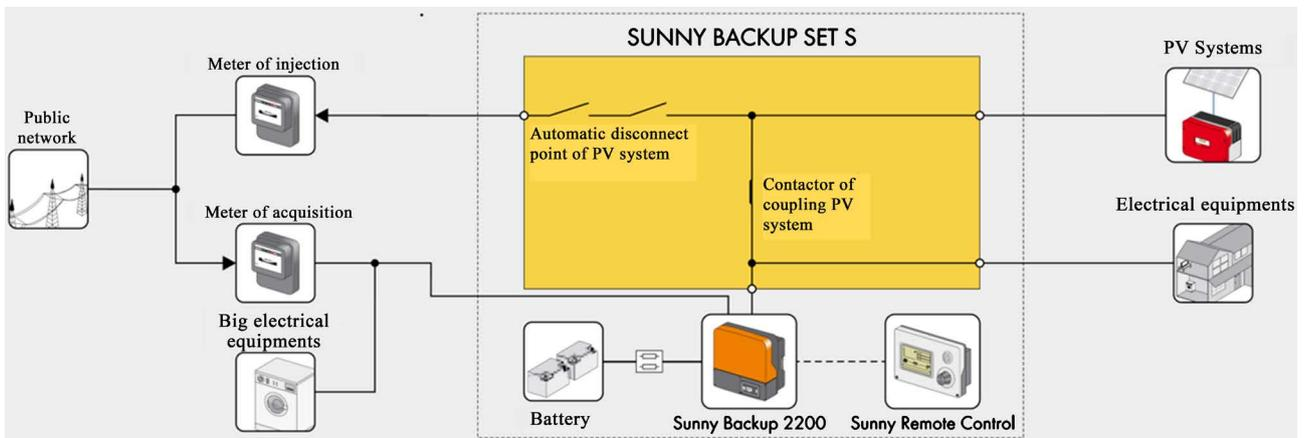
Figure 4. Functioning in autonomous mode.
