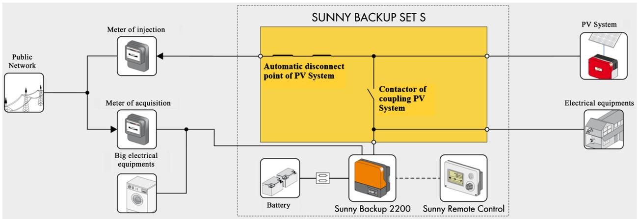
Figure 3. Functioning in injection mode.
