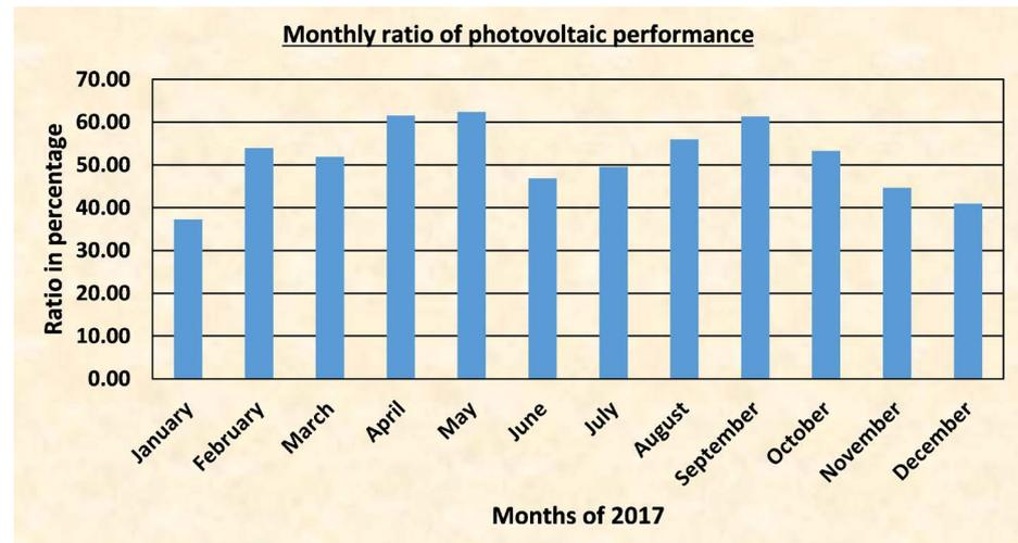
**Figure 8.** Monthly ratio of photovoltaic performance.
