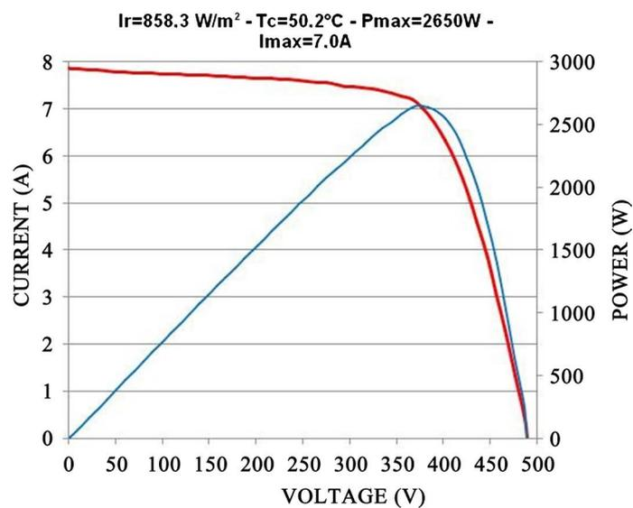
Figure 6. I/V characteristic curve.
