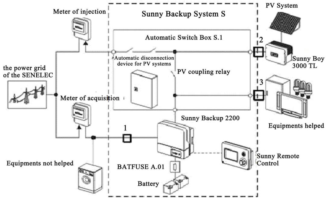
Figure 2. Plan of the installation.
