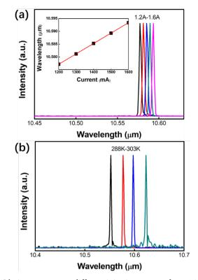
**Figure 2.** (a) CW lasing spectra at a different injection current from 1.2 to 1.6 A with a step of 0.1 A. The inset shows the linear-fit tuning characteristics of the lasing wavelength with electrical power for the same device. (b) CW emitting spectrum of QCL at different heat sink temperature between 288 and 303 K.
