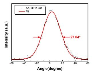
**Figure 4.** Measured lateral far-field radiation patterns for the devices at pulsed driving currents of 1 A under 5 kHz repetition frequency and 1% duty circle, the dot is the measurement and the red dashed line is the result fitted with the Gauss function.
