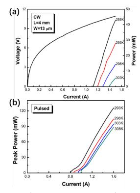
**Figure 1.** (a) Output optical power versus injection current of a 13  $\mu$ m-wide and 4-mm long device in CW mode at different heat sink temperatures between 288 and 303 K along with V-I curves at 288 K. (b) Peak power of the laser changes with heat sink temperatures at the repetition frequency of 5 kHz and a pulse width of 2  $\mu$ s.
