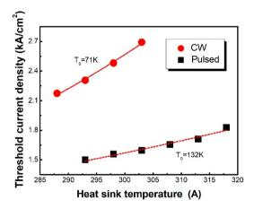
**Figure 3.** Threshold current density as a function of heat sink temperature in CW and pulsed mode of a 4-mm-long and 13- $\mu$ m-wide LWIR QCL. The red dashed line is fitted with the exponential function  $J_{th} = J_0 \exp(T/T_0)$ .
