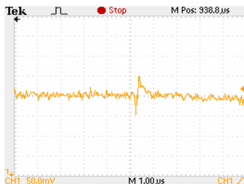
Figure 5. Response of transient load regulation((X-axis 1us/div, Y-axis 50mV/div)
