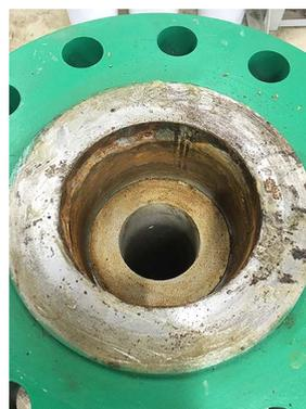
**Figure 15.** Helidon Sandstone cylinder (94 mm ID) within a 173.1 mm ID pipe after hydraulic testing. The sandstone cylinder was installed using a high tensile and flexural strength, low viscosity epoxy resin.
