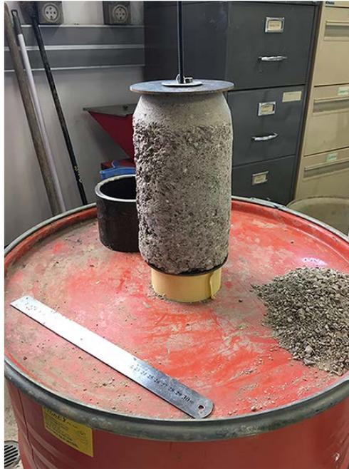
**Figure 10.** Originally 139.7 mm OD, stripped to 127 mm OD for the long term testing in the 139.8 mm ID pipe sections.
