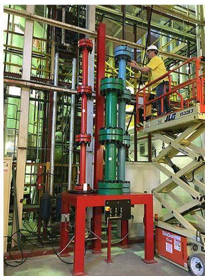
**Figure 2.** The Well Simulator Facility at the University of Queensland. Three different pipe sizes can be installed and tested up to a maximum pressure of 6.9 MPa (1000 psi). Sections of up to 5 m height can be installed. One pressure transducer is installed at the flange of each pipe and allow pressure monitoring while pumping.
