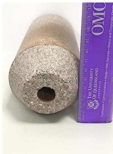
**Figure 1.** Bentonite plug with a diameter of 88.9 mm (3.5") and 190 mm length (7.5"). The central hole is 19 mm (0.75") wide.
