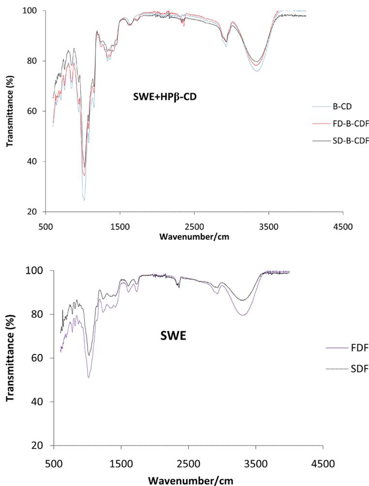
**Figure 9.** FTIR-spectra of HP $\beta$ -Cyclodextrin (B-CD), spray dried HP $\beta$ -Cyclodextrin with SWE (B-CD-SDF), Freeze dried HP $\beta$ -Cyclodextrin with SWE (FD-B-CDF), spray dried SWE (SDF) and Freeze dried SWE (FDF).
