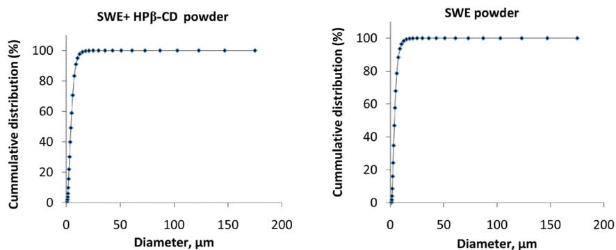
**Figure 3.** Cumulative distribution of particle size percent vs the upper limit of each size class from the HELOS and RODOS particle size analyser using density values of  $1.50 \text{ g/cm}^3$  (SWE + HP $\beta$ -CD powder) and  $1.56 \text{ g/cm}^3$  (SWE powder).
