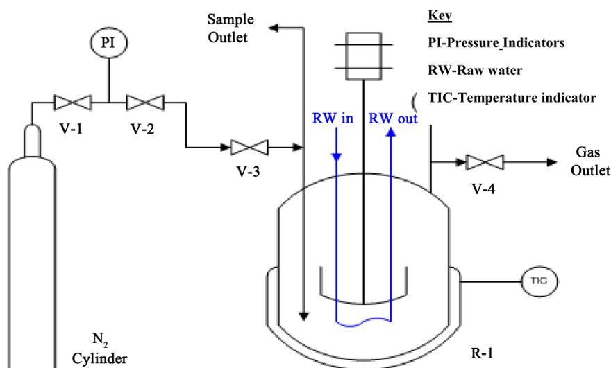
**Figure 1.** Setup for the subcritical water extraction of Apple pomace.
