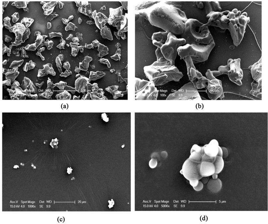
**Figure 4.** SEM images of freeze dried encapsulated phenolic fraction with natural polysaccharides co-extracted under subcritical water extraction of apple pomace (SWE); with Magnifications; (a) =50×; (b) =100×; (c) =1000× and (d) =5000×.
