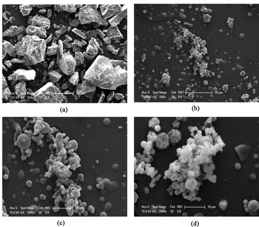
**Figure 7.** SEM images of freeze dried encapsulated subcritical water extract of apple pomace with HP-β-Cyclodextrins (SWE + HP-β-CD); with Magnifications; (a) =100×; (b) =500×; (c) =1000× and (d) =2000×.
