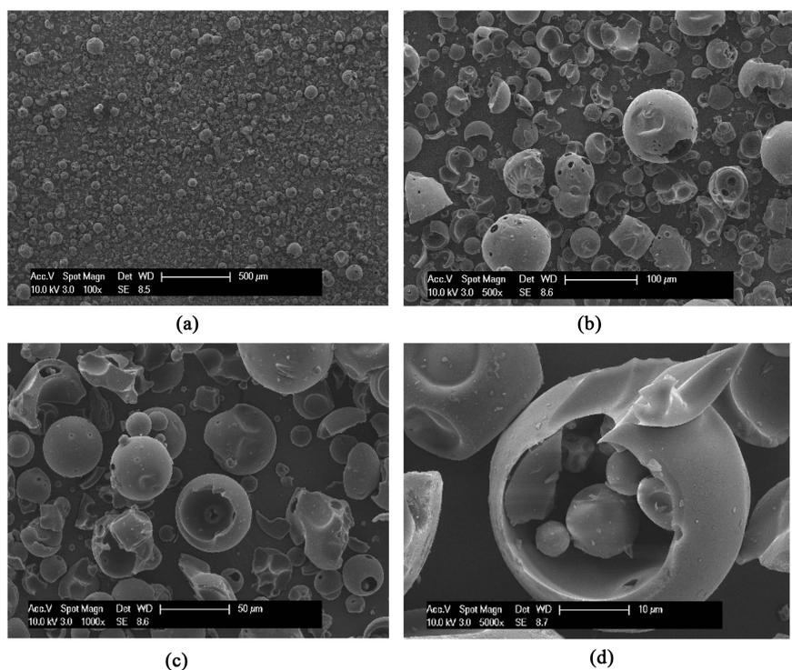
**Figure 6.** SEM images of pure HP-β-Cyclodextrins Powder with magnifications; (a) =100×; (b) =500×; (c) =1000× and (d) =5000×.
