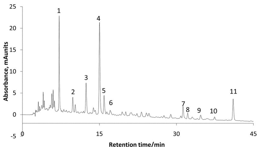
**Figure 11.** Chromatogram of subcritical water extract (SWE) at 150 °C for 30 minutes; 1: 5HMF; 2-furfural, 3: Protocatechuic aldehyde; 4: Chlorogenic acid; 5: (isomer of Chlorogenic acid); 6: caffeic acid; 7: Quercetin-3-galactoside; 8: Quercetin-3-glucoside, peak 9 and 10 not identified; 11: Phlorodzin.
