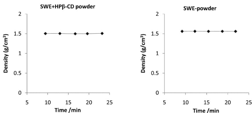
**Figure 2.** The density of powder as a function of time under 5 cycles with purge fill pressure of 19.50 psig and equilibrating rate at 0.020 psig per minute.
