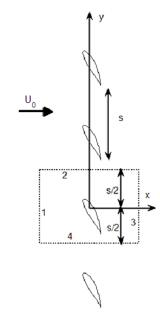
Figure 1. Control volume for cascade of equi-spaced identical bodies.
