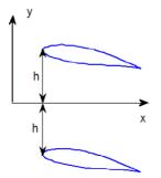
Figure 4. Aerofoils comprising a biplane. Control volume as in Figure 3.
