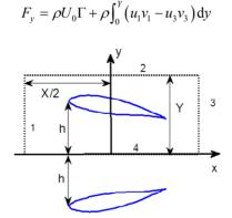
Figure 3. Aerofoil in ground effect.
