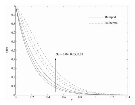
Figure 5. Velocity profiles for variations in Da when Pr = 0.71, Gr = 25,  $\tau = 0.1$  and Ra = 2.
