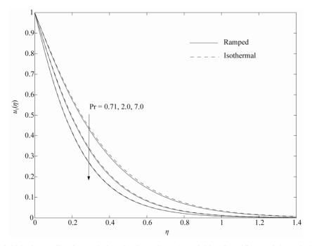
Figure 3. Velocity profiles for variations in Pr when Da = 0.04, Gr = 25,  $\tau = 0.1$  and Ra = 2.
