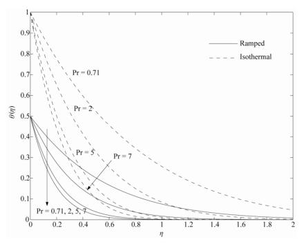
Figure 8. Temperature profiles for variations in Pr when Ra = 2 and  $\tau = 0.5$ .
