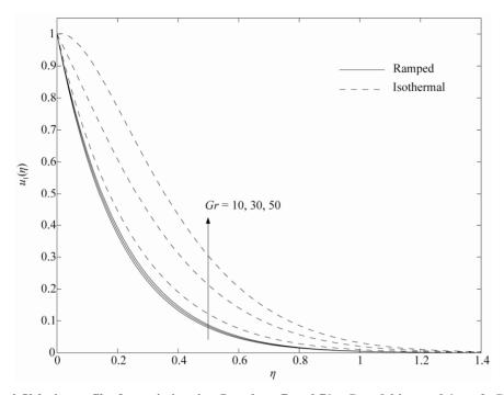
Figure 4. Velocity profiles for variations in Gr when Pr = 0.71, Da = 0.04,  $\tau = 0.1$  and Ra = 2.
