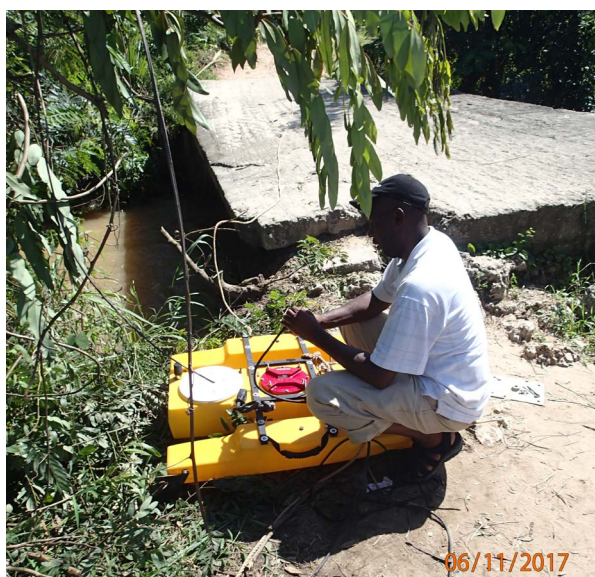
Figure 9. WRA Officer deploying ADCP equipment downstream of the KISCOL weir.
