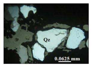
**Figure 9.** Photo micrograph showing the shape of quartz under the polarizing microscope (Qz: quartz).
