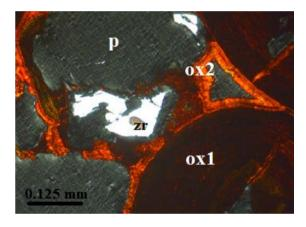
**Figure 8.** Photo micrograph showing the oxides and hydroxides seen under the polarizing microscope (Ox1: oxides and hydroxides forming mostly oolites and pisolites cortex, Ox2: oxides and hydroxides forming mostly the binding agent, P: pores, Zr: zircon).
