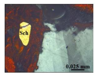
**Figure 11.** Photo micrograph showing the scheelite highlighted in ferruginous sandstones, under the polarizing microscope (Sch: scheelite).
