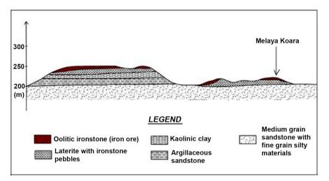
**Figure 4.** Cross section of the Tourougo area showing the vertical succession of the Continental Terminal deposits. The uppermost deposits include the oolitic iron mineralisation (Location in **Figure 2**).
