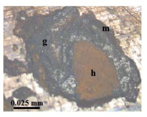
**Figure 12.** Photo micrograph showing different oxides and hydroxides observed in polished section (g: goethite, h: hematite, m: magnetite).
