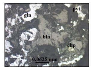
**Figure 13.** Photo micrograph showing different sulphides observed in polished section (gln: galena, bln: blende, pyt: pyrite, chp: chalcopyrite).
