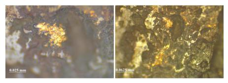
Figure 14. Photo micrograph showing gold observed under the metallographic microscope.
