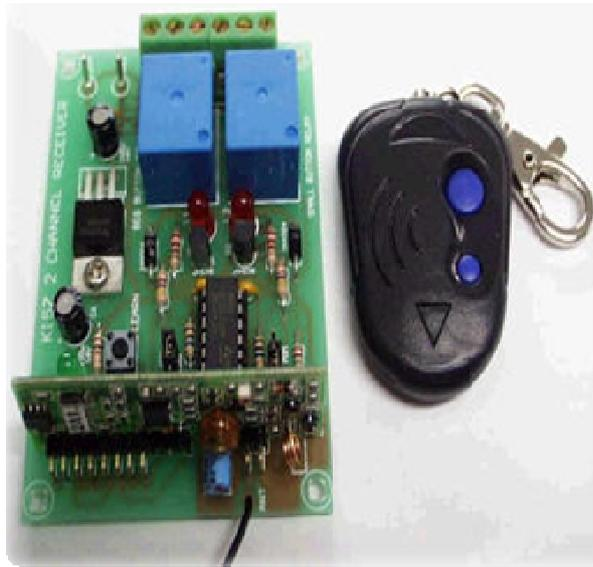
Figure 5. Relay receiver board with remote control.
