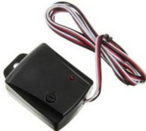
**Figure 1. Vibration detector alarm sensor AK-CGQ.**
