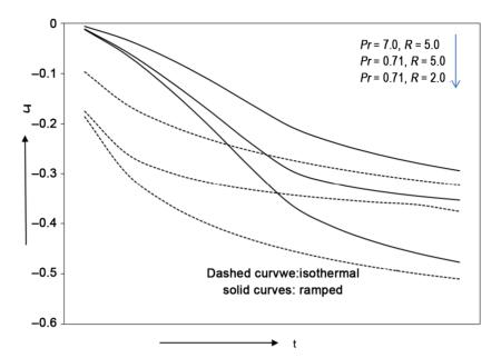
Figure 8. Variation of skin friction for ramped and isothermal temperature.
