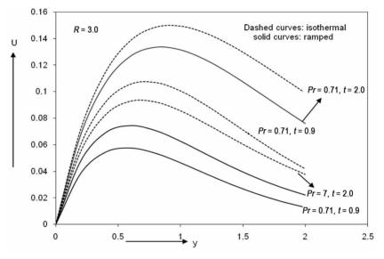
Figure 4. Velocity profile for different Pr and t.
