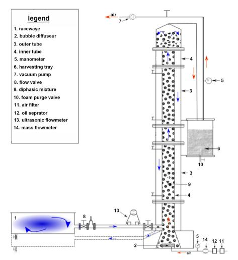
Figure 1. Experimental setup.
