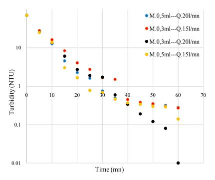
**Figure 2.** Clay particles extraction with MIBC + casein (0.014 g·l<sup>-1</sup>).
