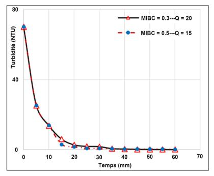
Figure 4. Efficacity of clay particles extraction by combined MIBC and casein.
