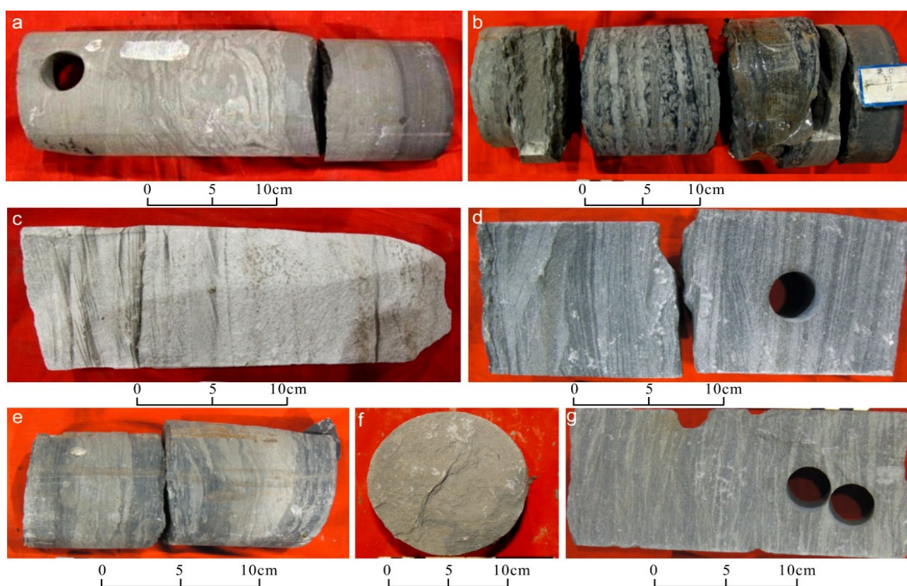
Figure 2. The sedimentary characteristics of Qingshankou to Yaojia Formation in West Slope Area. (a) Siltstone, deformation bedding, gravity flow deposition, First Member of Qingshankou Formation, Well Y51; (b) Thin interlayer of sandy mudstone, liquefaction structure, Bouma sequence, gravity flow deposition, First Member of Qingshankou Formation, Well Y51; (c) Fine sandstone, one-way flow bedding, underwater distributary channel, First Member of Qingshankou Formation, Well D84; (d) Fine sandstone, parallel bedding, two-way flow bedding, mouth bar, Yaojia Formation, Well L31; (e) Deformation bedding, sheet sand, Second Member of Qingshankou Formation, Well G98; (f) Biotic mudstone, mouth bar, Yaojia Formation, Well D56; (g) Small trough cross-bedding, underwater distributary channel, Yaojia Formation, Well G844.
