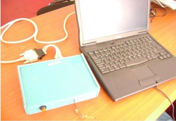
**Figure 3.** Diagram of a basal body temperature (BBT) logger interfaced with a personal computer.
