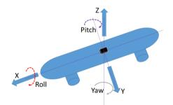
Figure 1. Accelerometer and gyroscope on skateboard.
