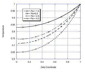
**Figure 4.** Dimensionless temperature profile for values of  $\psi$ .
