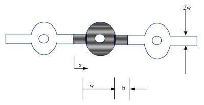
Figure 1. Schematic of fin pipe and radiative radial fin.
